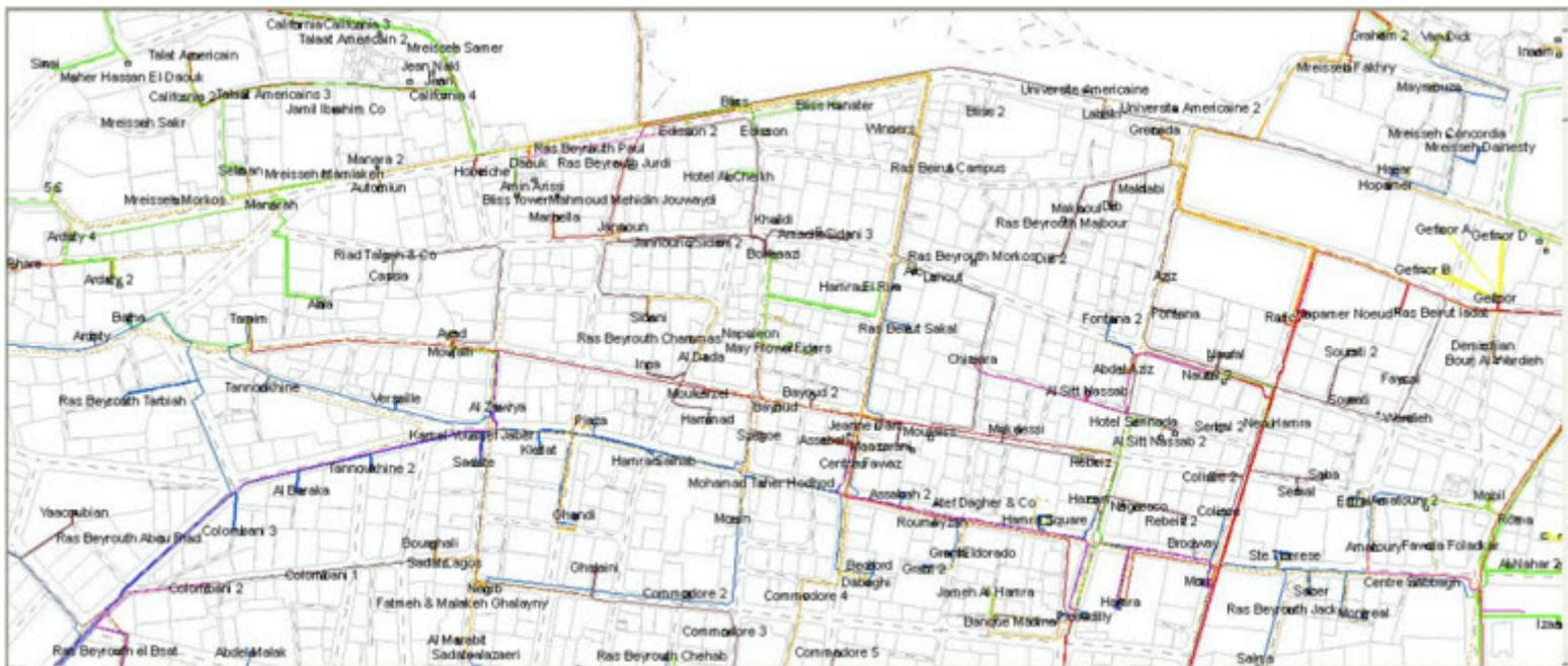
Figure 4. Electrical power network, colored by substation line. (Provided by EDL)
