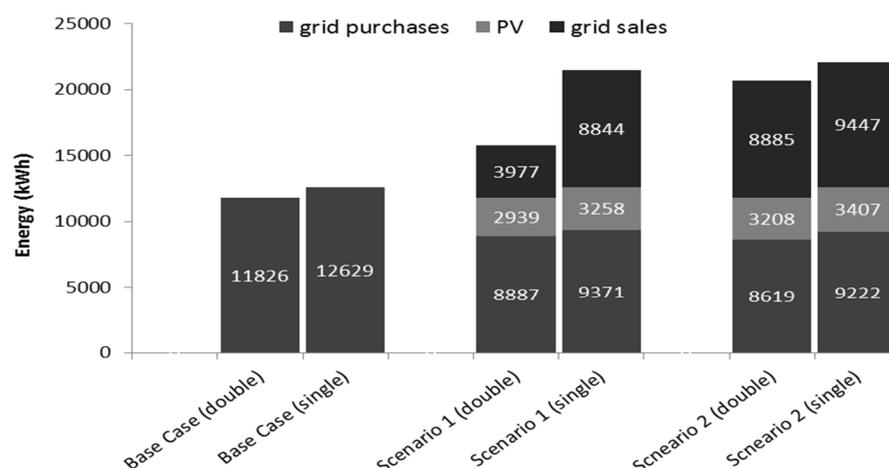
Fig. 6: Plot of grid purchases, electric load covered by the PV system, and grid sales for the Base case, Scenario 1, and Scenario 2 if single glazed or double glazed is used (grid sales constraint).
