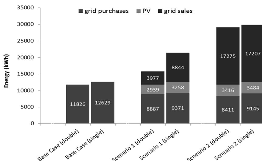
Fig. 5: Plot of grid purchases, electric load covered by the PV system, and grid sales for the Base case, Scenario 1, and Scenario 2 if single glazed or double glazed is used (no grid sales constraint).
