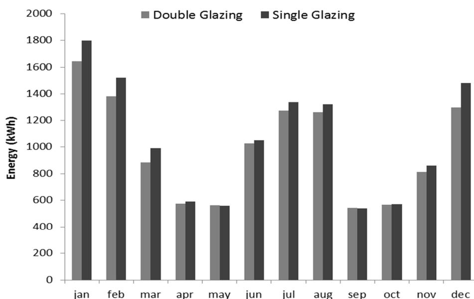
Fig. 3: Energy Consumption for each month when single glazing and double glazing are used
