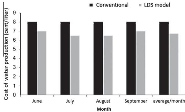
Fig. 7. The cost of water production in cent/liter for each of the cooling months from the LDS and conventional vapor compression commercial system.
