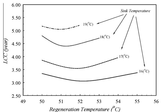
**Fig. 6.** The *LCC* as a function of regeneration temperature at different heat sink temperatures.
