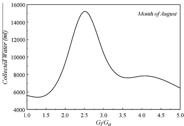
**Fig. 4.** The variation of the predicted collected water versus the liquid desiccant to air flow rate ratio of the designed system using six solar concentrators and  $1\text{ kg/s}$  of air flow for the month of August.
