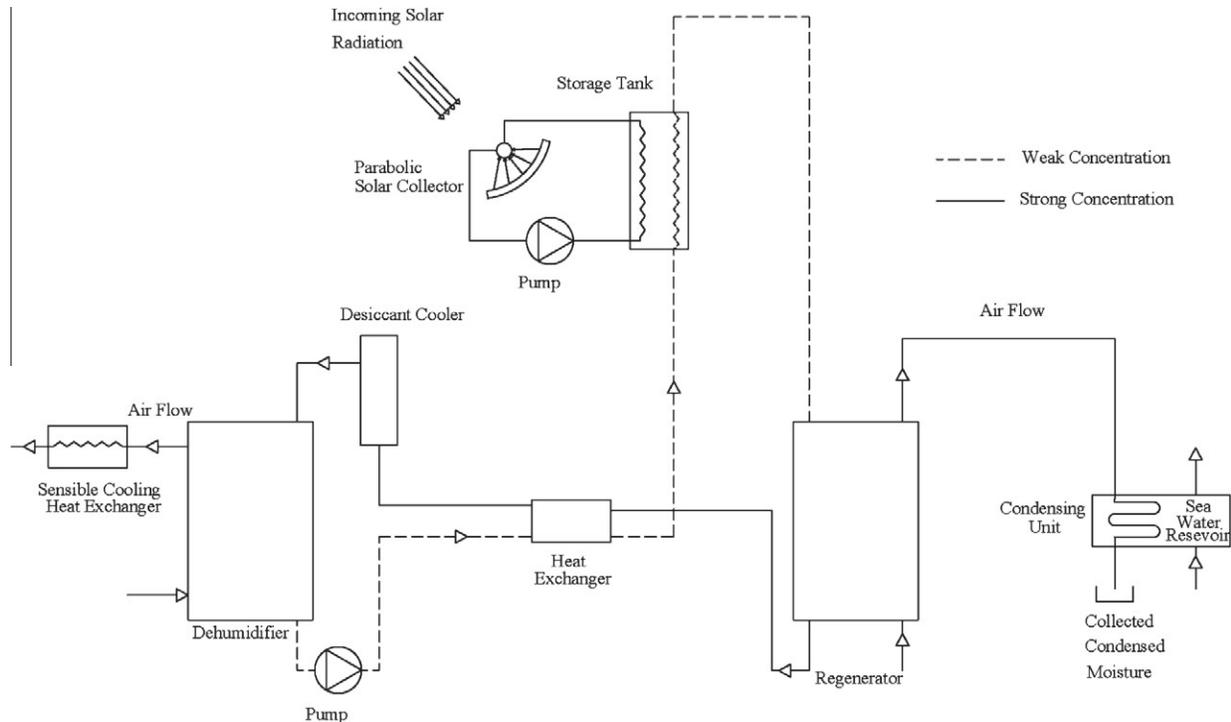
Fig. 1. Schematic of the liquid desiccant system.
