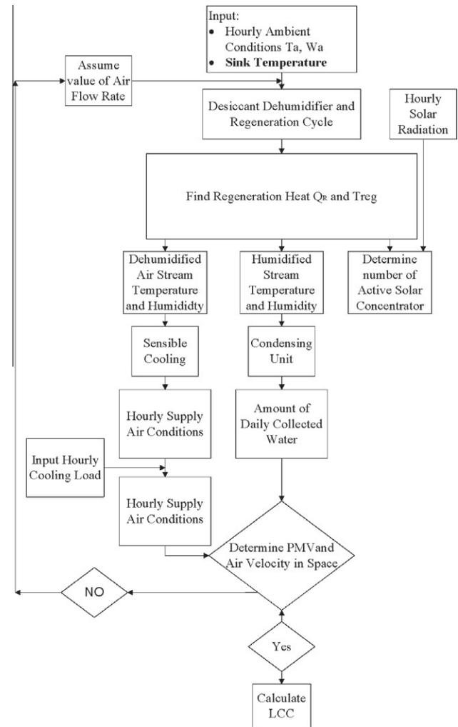
Fig. 2. Flow chart of the solution and optimization procedure.
