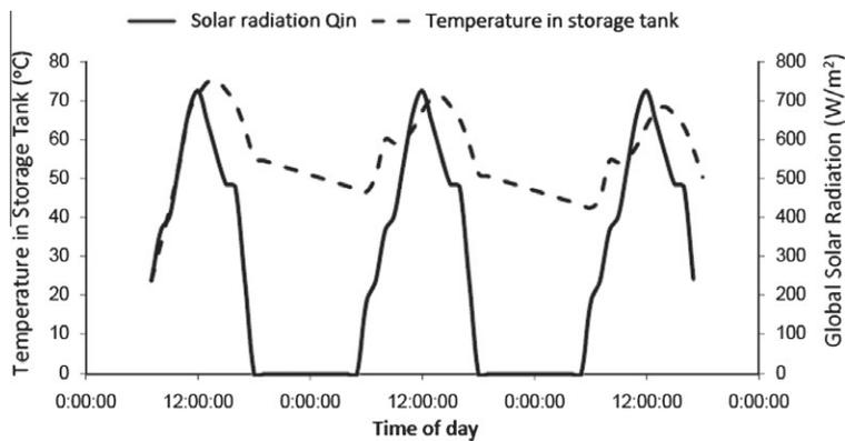
Fig. 5. The storage tank temperature and incident global solar radiation for typical August day in Beirut climate.
