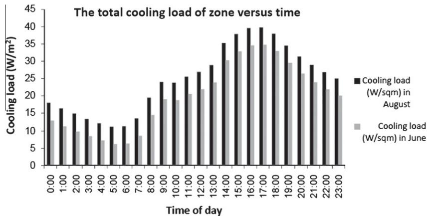
Fig. 3. The hourly cooling load for the months of June and August.
