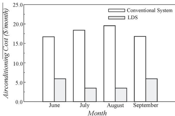
Fig. 8. The monthly cost of both the conventional and current proposed LDS.
