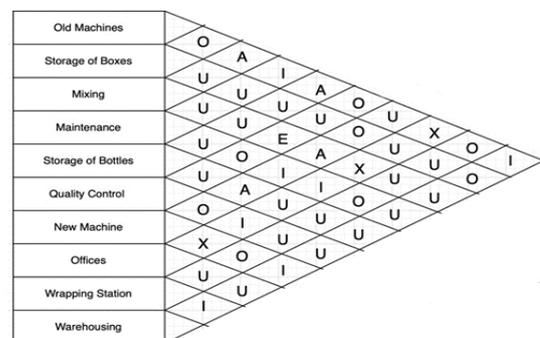
Fig. 4- Developed Activity Relationship Diagram
